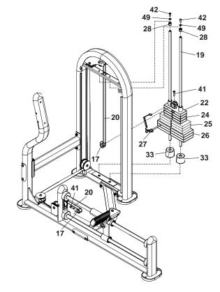
Install the top plate (22) on the weight stack guide posts (19), inserting the top plate shaft through the holes in the weights. Insert the selector pin (27) through one weight until it engages the top plate shaft.
